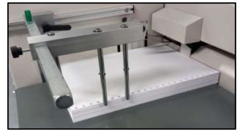
Feeder on the side of the machine with easy joggings adjustments
