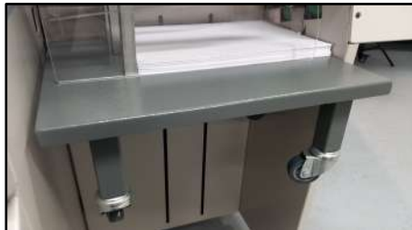
Receiving tray on wheels for easy movement of heavy loads by the operator
