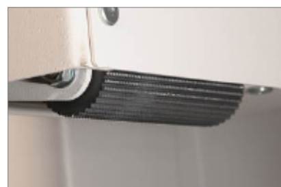
Improved PGO roughener for spine preparation, especially for difficult, thick, coated papers.
