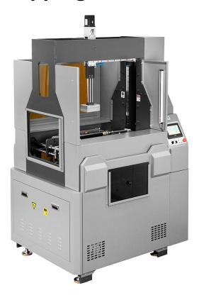
GC-420 is an automated machine dedicated to wrapping cover on a box made of solid cardboard. Machine is dedicated to small and medium volume. This is the latest version of the device where the external dimensions of the box (length, width, height) are entered on the touch screen - the machine automatically adjusts to the given dimension which makes it ideal solution for on demand production.
